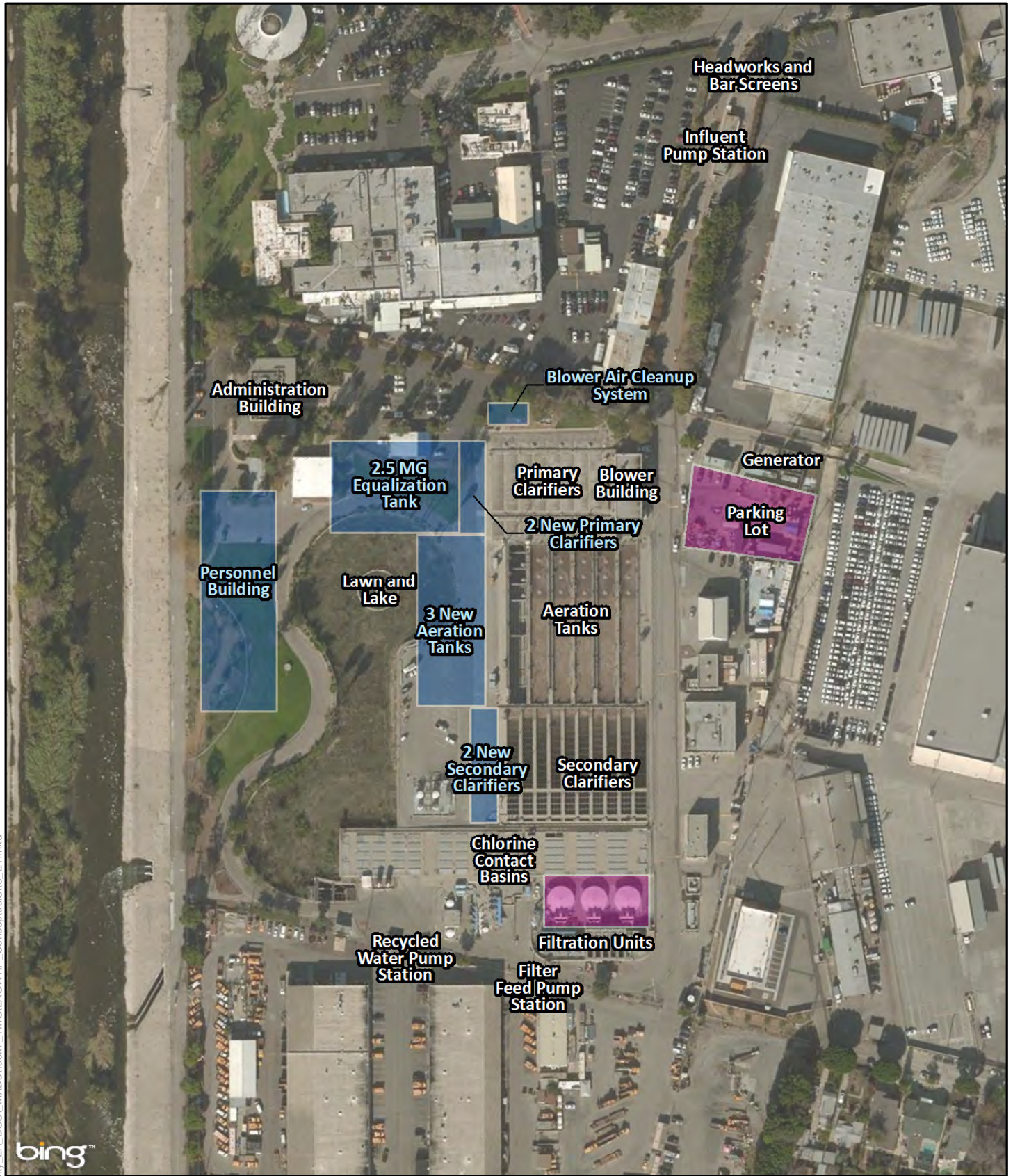
Figure 6.9 Potential Process Location for Concept Option #17 (LAGWRP to Headworks Reservoir) One Water LA 2040 Plan
