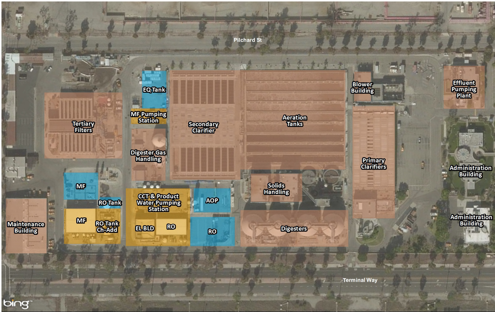
Figure 7.6 Site Layout for Phase 1 and Phase 2 AWP at TIWRP One Water LA 2040 Plan
