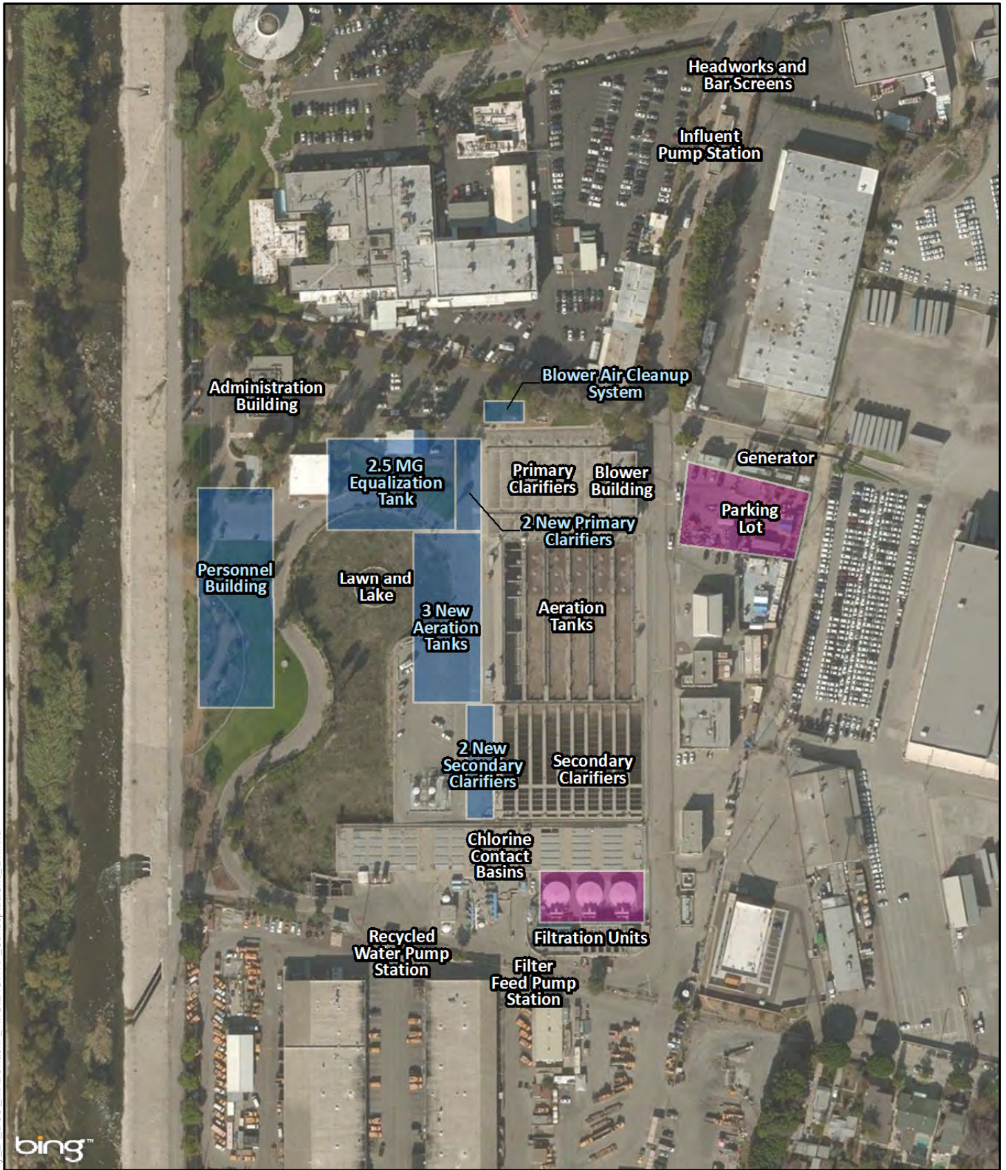
Figure E.4 Potential Process Location for Concept Option #17 (LAGWRP to Headworks Reservoir) One Water LA 2040 Plan
