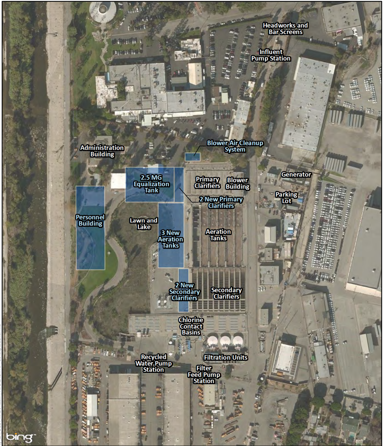
Figure 6.5 LAGWRP Primary Effluent Equalization Storage One Water LA 2040 Plan
